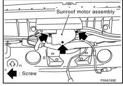
6. Remove nuts on the front end and side rail.
